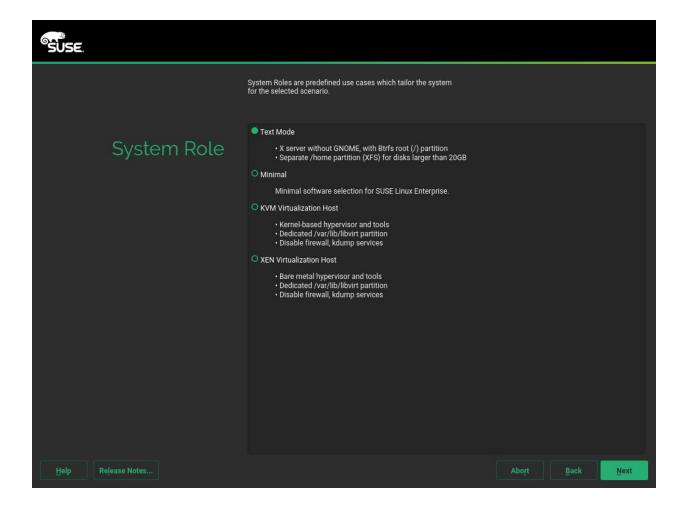
The availability of system roles depends on your selection of modules and extensions. System roles define, for example, the partitioning proposal and the set of software patterns that is going to be preselected for the installation. Refer to the description on screen to make your choice. Select a role and proceed with *Next*.
