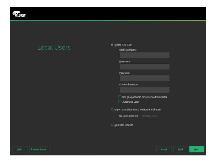
To create a local user, type the first and last name in the *User's Full Name* field, the login name in the *Username* field, and the password in the *Password* field.
