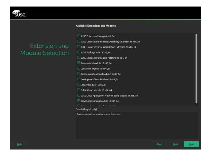
After the system is successfully registered, the installer lists modules and extensions that are available for SUSE Linux Enterprise Server. Modules are components which allow you to shape the product according to your needs. They are free of charge. Extensions add functionality to your product. They are offered as subscriptions and require a registration key that is liable for costs.
