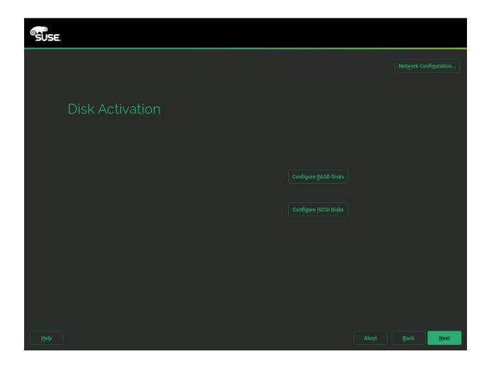
Configure the attached hard disks. Select DASD, Fibre Channel Attached SCSI Disks (zFCP), or iSCSI for the installation of SUSE Linux Enterprise Server. The DASD and zFCP configuration buttons are only available if the corresponding devices are attached. Proceed with *Next* to set up the selected disk type.
