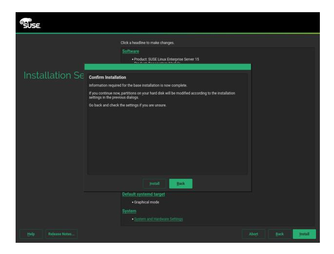
After you have finalized the system configuration on the *Installation Settings* screen, click *Install*. Depending on your software selection you may need to agree to license agreements before the installation confirmation screen pops up. Up to this point no changes have been made to your system. After you click *Install* a second time, the installation process starts.
