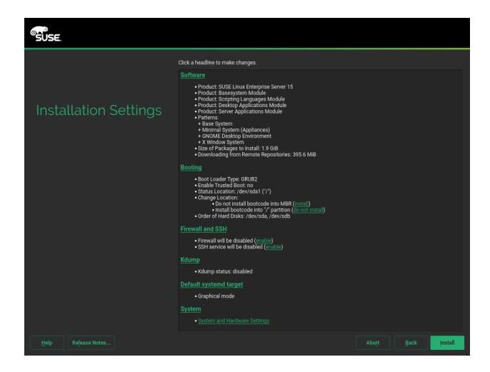
Use the *Installation Settings* screen to review and—if necessary—change several proposed installation settings. The current configuration is listed for each setting. To change it, click the headline. Some settings, such as firewall or SSH can directly be changed by clicking the respective links.
