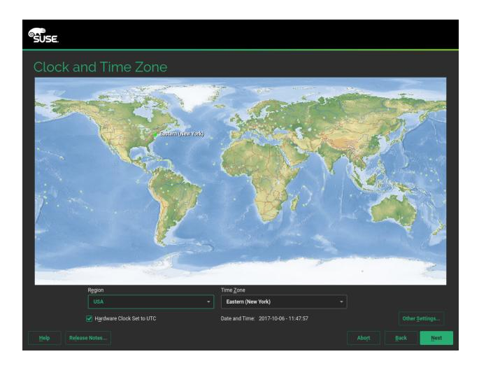
Select the clock and time zone to use in your system. To manually adjust the time or to configure an NTP server for time synchronization, choose *Other Settings*. See *Book "*Deployment Guide", *Chapter 8 "Installation Steps"*, *Section 8.12 "Clock and Time Zone"* for detailed information. Proceed with *Next*.
