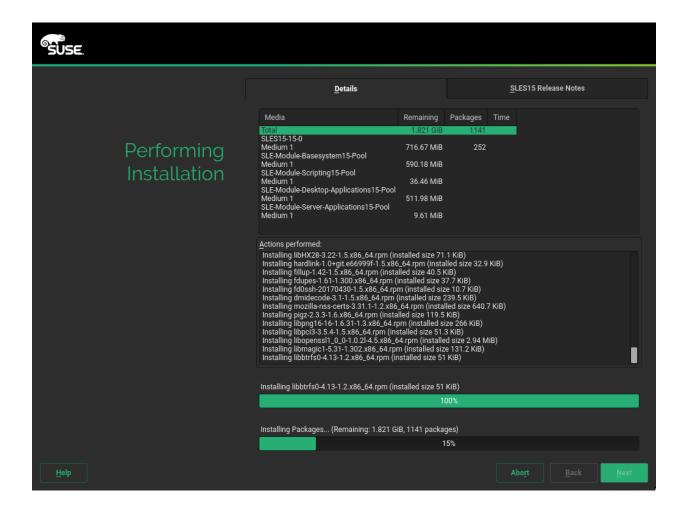
During the installation, the progress is shown in detail on the *Details* tab.
